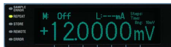
High resolution output with ±120,000 display counts and 100 nV steps minimum
