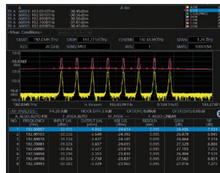
Figure 3 – The automated routine for the analysis of optical amplifiers provides a table with their relevant parameters
