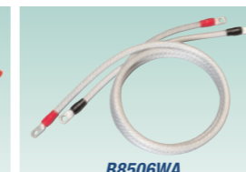
B8506WA Measurement lead set 2 pieces (red and black) in 1 set, length : 1.5 m, Rating : 80 A
