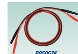
B8506ZK Measurement lead set 2 pieces (red and black) in 1 set, length: 1.00 m Used in combination with the B8506ZL, 701902, 758921, 758922, or 758929. Rating: 1500 V CAT I/19 A
