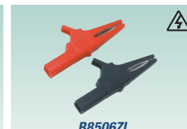
B8506ZL Large Alligator clip adapter set Safety terminal (banana female)-to-alligator clip adapter 2 pieces (red and black) in 1 set Rating: 1500 V CAT I Connected to the B8506ZK, 758933, 758917, or 701901.
