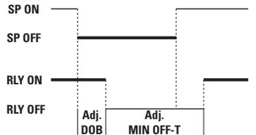
When the signal deactivates the setpoint, the relay remains energized until the programmable DOB period times out.
