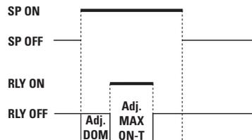
When the signal activates the setpoint, the DOM prevents the relay from energizing until the programmable DOM setting times out.
