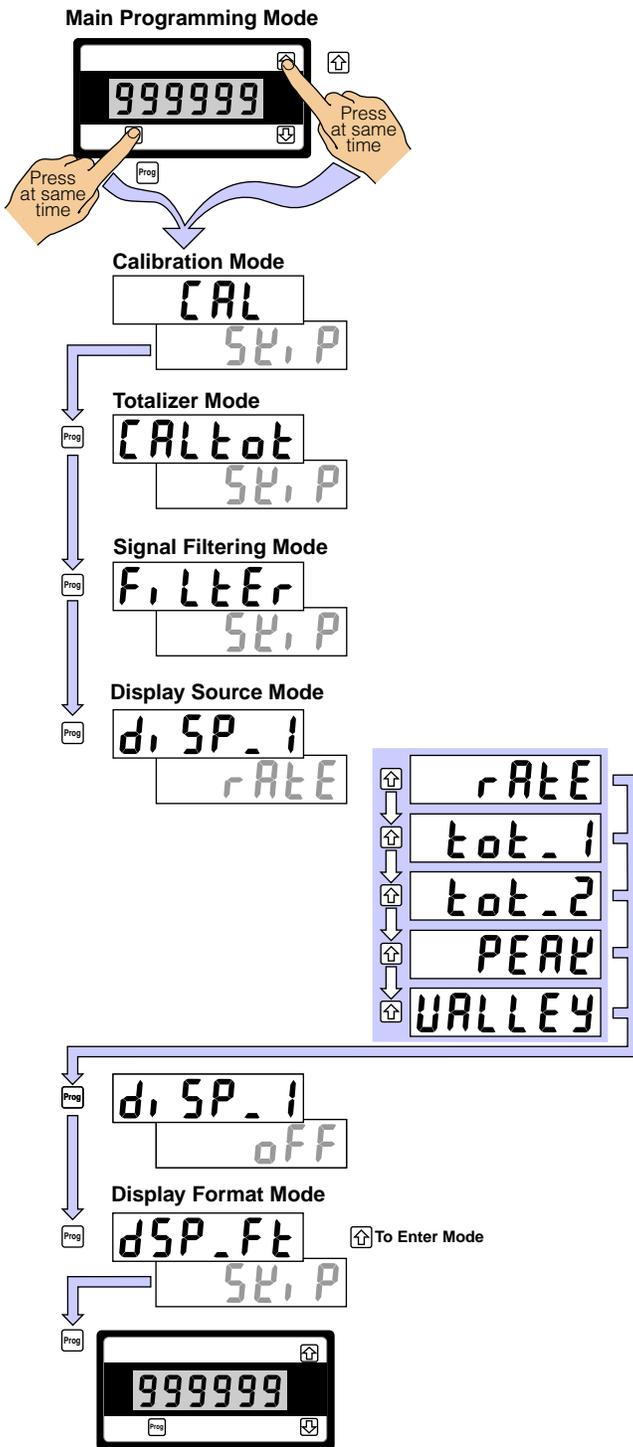
The **display source mode** allows you to select the source for the operational display. This means that any one of the following can be displayed on the operational display while the rest can be viewed on the recall display of the view mode by simply pressing the  $\uparrow$  or  $\downarrow$  button:
