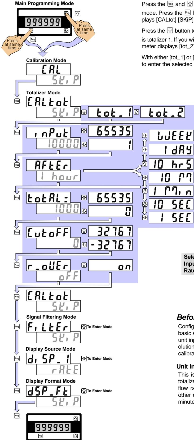
Press the **Prog** and **↑** buttons at the same time to enter the main programming mode. Press the **Prog** button again to skip the calibration mode. The meter displays [CALtot] [SKiP]. This is the **totalizer mode**.
