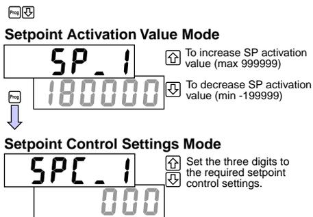
While programming, pressing the **Prog** button saves the current programming settings and moves on to the next programming step or mode.
