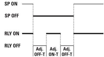
In this mode the off-time setting activates first. When the signal deactivates the setpoint, the relay remains de-energized for the programmed OFF-T setting and energizes when the ON-T setting activates.
