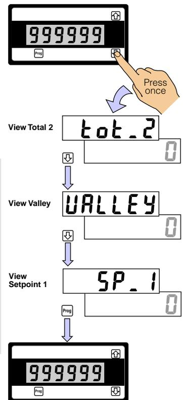
**Note:** While in the **total 2** view mode, pressing the Up and Down buttons at the same time resets totalizer 2 to 0 (zero).
