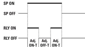
In this mode the on-time setting activates first. When the signal activates the setpoint, the relay energizes immediately and remains energized for the programmed ON-T setting.
