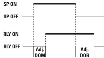
When the SP deactivates, the DOB delay keeps the relay energized for the programmed time period.
