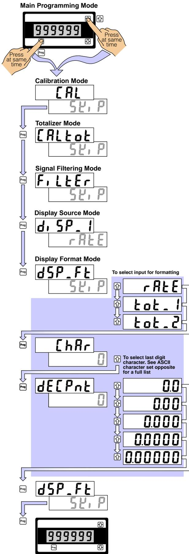
The **display format mode** allows you to format how the input signal (rate), total 1, and total 2 are displayed when shown on the operational or recall displays.
