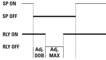
The OFF-T then de-energizes the relay for the MAXIMUM programmed off-time period.
