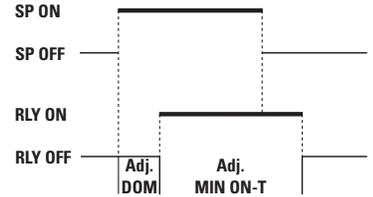
When the signal activates the setpoint, the DOM prevents the relay from energizing until the programmable setting times out.
