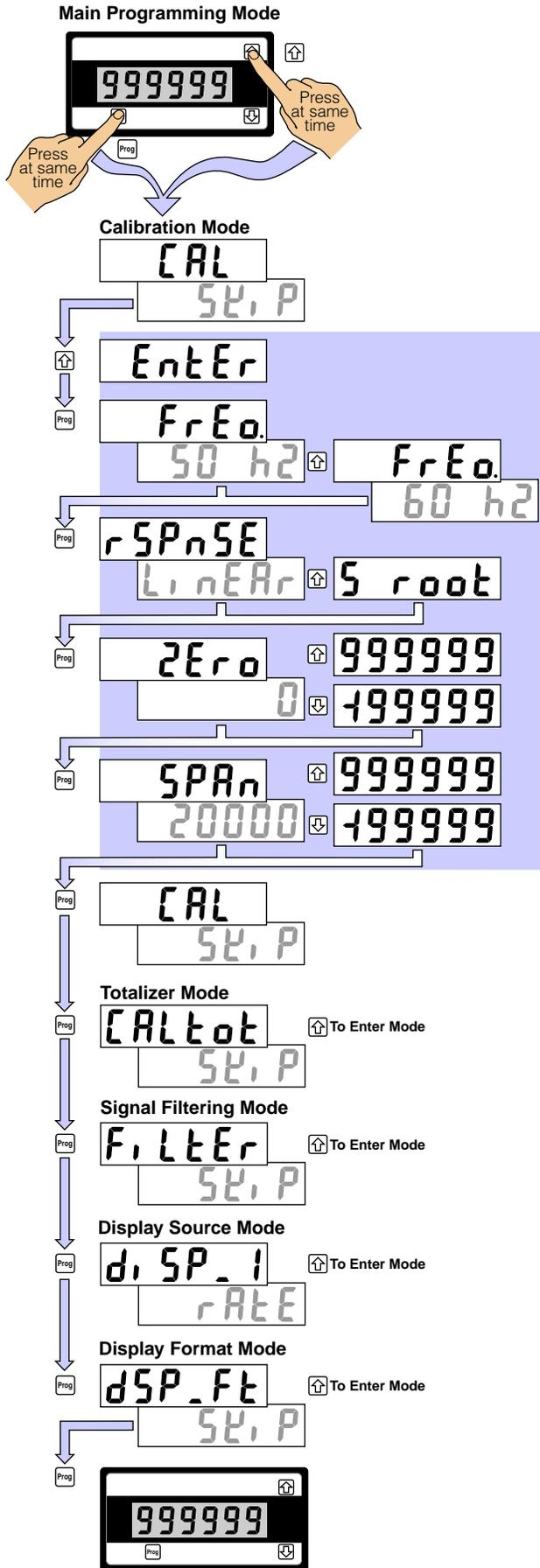
Press the **Prog** and **Up** buttons at the same time to enter the **main programming mode**. The **calibration mode** is the first mode that appears. It allows you to:
