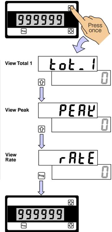
**Note:** While in the **total 1** view mode, pressing the Up and Down buttons at the same time resets totalizer 1 to 0 (zero).
