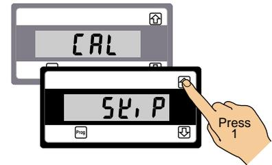
Where a left and right hand are shown on separate buttons on the same diagram, this indicates that the buttons must be pressed at the same time.
