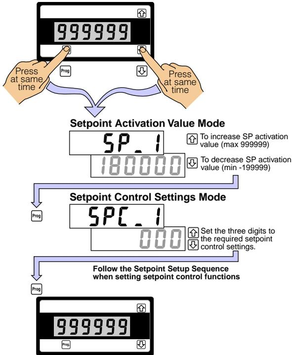
All setpoint activation and control settings are selected and configured using the front panel buttons in the **setpoint programming mode**. The meter has one software driven setpoint configured to operate within the total span range of the meter.
