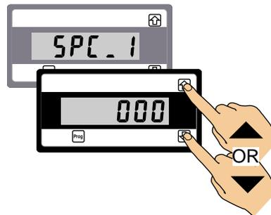
When two displays are shown together as black on grey, this indicates that the display is toggling (flashing) between the name of the function and the value or configuration setting.
