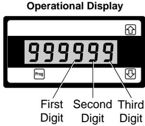
To explain software configuration procedures, diagrams are used to visually describe the programming steps. The following conventions are used to represent the buttons and indicators on the meter, and the actions involved in programming the meter:
