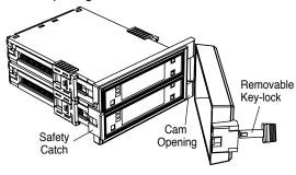
Clear Lockable NEMA 4X Splash Proof Cover can accept two 1/16 DIN cases P/N:(OP-N4/96x48)
