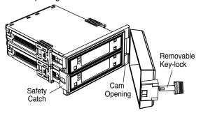
Clear Lockable NEMA 4X Splash Proof Cover can accept two 1/16 DIN cases P/N:(OP-N4/96x48)
