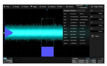
The Waveform Histogram feature provides a statistics view of the waveform in horizontal and vertical directions
