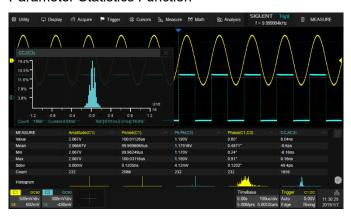
Statistics shows the current value, maximum value, minimum value, standard deviation and mean value of up to 12 parameters simultaneously. Histogram is available to show the probability distribution of a parameter. Trend is available to show the parameter value vs. time
