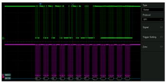
Display the decoded characters through the events list. Bus protocol information can be quickly and intuitively displayed in tabular form. I<sup>2</sup>C, SPI, UART, CAN, LIN, CAN FD, FlexRay, I<sup>2</sup>S, MIL-STD-1553B, SENT, Manchester and ARINC 429 are supported
