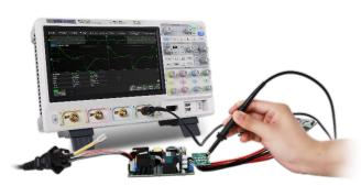
The SDS5000X can control the USB AWG module or a standalone SIGLENT SDG generator, to scan the amplitude and phase frequency response of the DUT, and display the data as a Bode Plot. This makes it possible to replace expensive network analyzer in some applications The Power Analysis option provides a full suite of power measurements and analysis, which greatly improve the measurement efficiency in switching power supplies and power devices design
