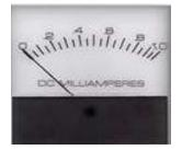
Traditional square meters with the look of the 80s and a low price tag, these have operating zero adjusters and scales printed on translucent plastic, permitting diffused back-lighting using either the external light kit described in "Options" or custom lighting. Installation holes and cutouts are interchangeable with domestic and foreign designs, making product improvement quick and easy.
