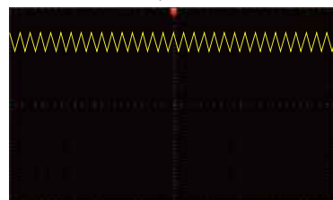
DC+AC Vdc=50V, triangle ripple Vac=5V, frequency 150Hz
