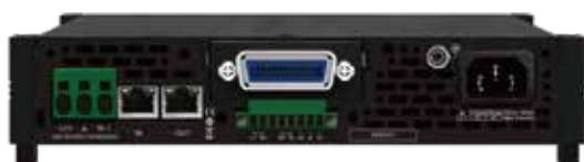
Rear panel with optional interface IT-E1208
