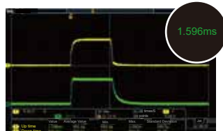
8 sets of IT6522C paralleling together Voltage ratings: 10V Current ratings: 960A Load current: 800A
