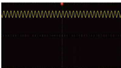
DC+AC Vdc=50V, sine ripple Vac=5V, frequency 150Hz
