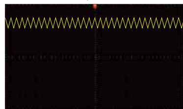
DC+AC Vdc=50V, triangle ripple Vac=5V, frequency 150Hz
