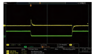
8 sets of IT6522C paralleling together Voltage ratings: 10V Current ratings: 960A Load current: Level A=100A Level B=800A F=10Hz
