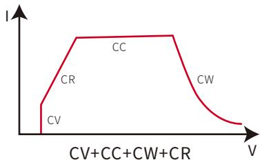
CV+CC+CW+CR mode can be applied to test lithium-ion battery charger, to gain complete V-I charging curve.In addition, when protection circuit of DUT is damaged, it can auto switch to avoid damage.
