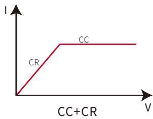
CC+CR mode is normally applied in the testings of OBC voltage limit, current limit characteristics, constant voltage and current accuracy testing, so as to prevent OBC over current protection.
