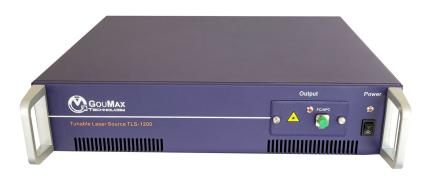
GouMax's TLS-1200 tunable lasers are new-generation high performance continuous wave (CW) tunable laser sources for use in various single band or combined band windows, ranging from 1050 nm to 1680 nm. The innovative design employs the state-of-the-art tunable technology and gain continuation in wide wavelength range. With no moving parts, the voltage-controlled wavelength tuning enables rapid wavelength switching over the whole operating wavelength window.
