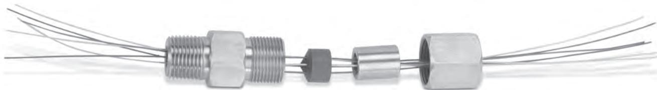
Conax Technologies BSWS assemblies were originally designed for use with embedded bearing temperature sensors to prevent oil migrating along the sensor leads. They seal on the individual insulated leads exiting an oil-filled bearing house. They may also be used to seal all types of insulated instrumentation leadwire. These sealing assemblies can be found in large motors, generators, turbines, pumps, compressors and journal bearing pedestals.
