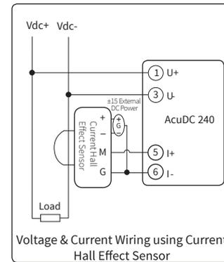
**NOTE:** Hall effect sensor can also be powered using the ±15V power supply in the X5 module.
