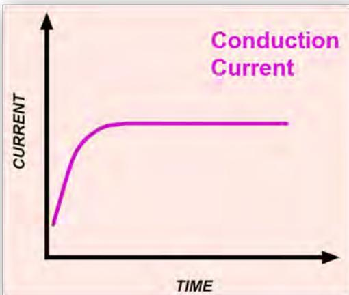
Conduction current, often called leakage current, is the steady current present both through and over the insulation.
