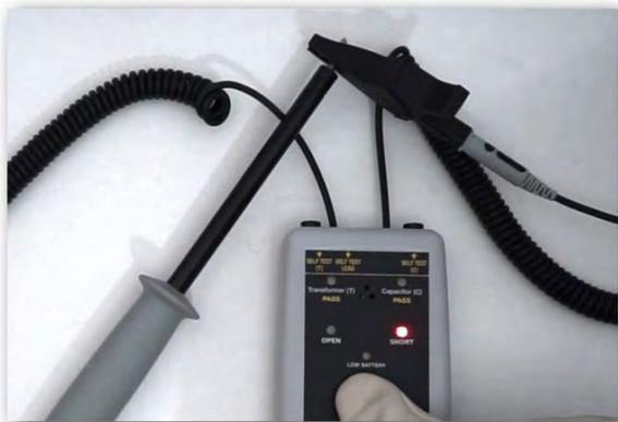
6. Separate the probe from the clip. Insert the tip of the probe into the terminal labeled SELF TEST (T), and then press the TEST button. The green Transformer PASS light should blink, and the buzzer should emit a steady sound.
