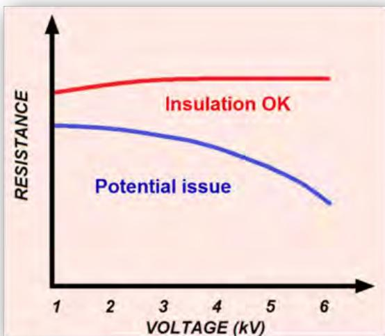
The Step Voltage test is designed to create electrical stresses on internal insulation cracks, identifying potential problems that may not be revealed by testing at lower voltages. Insulation that is thoroughly dry, clean, and in good physical condition should provide roughly the same resistance measurements across the voltage range. If instead you observe a significant
