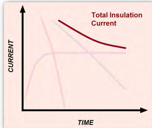
Understanding how these individual currents contribute to the total insulator current can help you correctly interpret the results you receive when performing a test.
