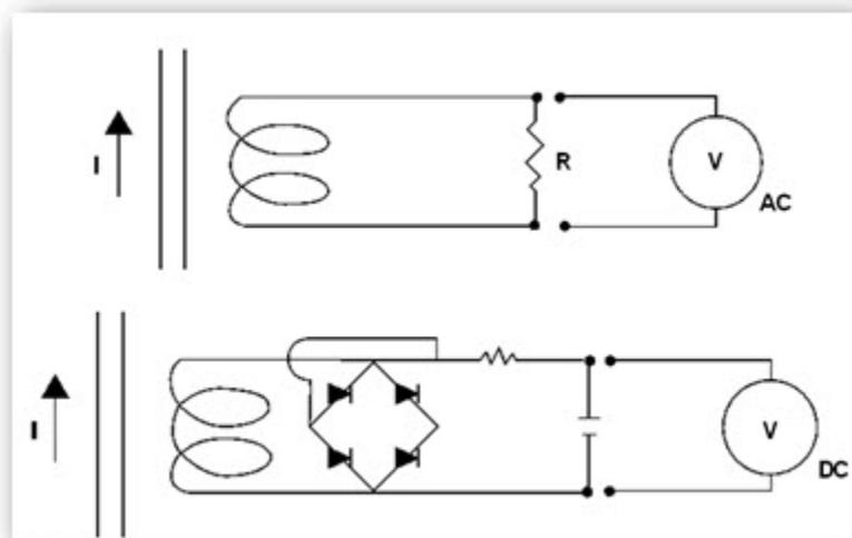
This is simply done by conditioning the current probe output inside the probe to provide voltage (e.g., Model MN251). In these cases, the probe mV output is proportional to the measured current (e.g., 1mVAC/AAC).
