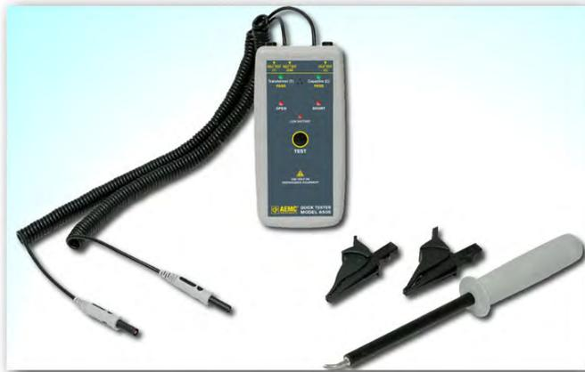
The AEMC® Quick Tester Model 8505 is a hand-held instrument for performing basic integrity tests on transformers and capacitors used by manufacturers and electrical utilities. This instrument is a fast and inexpensive inspection tool for detecting opens or shorts caused by shipping damage or workmanship issues.
