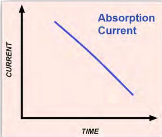
This gradual change reflects the storage of potential energy in and along the insulation. As a result, resistance is initially lower and then rises. This produces a measurement profile similar to capacitive charging current, but at a much slower rate; the effect can last from several seconds up to a minute or more.
