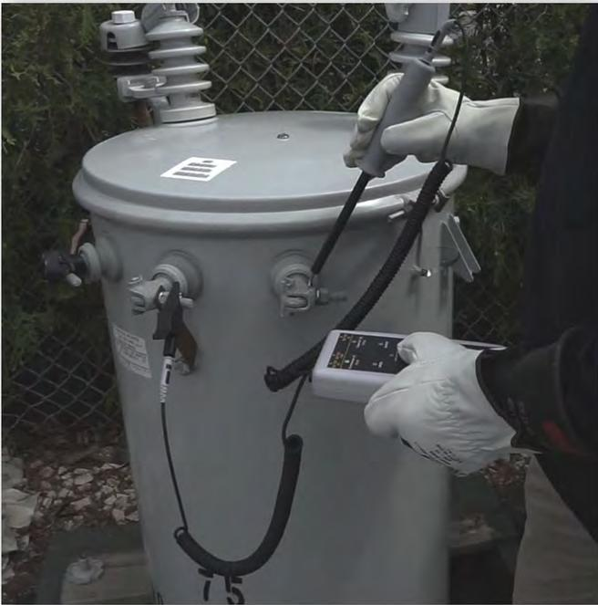
Turn the secondary circuit breaker to the off position, and repeat these tests. In each test, the red OPEN light should blink.
