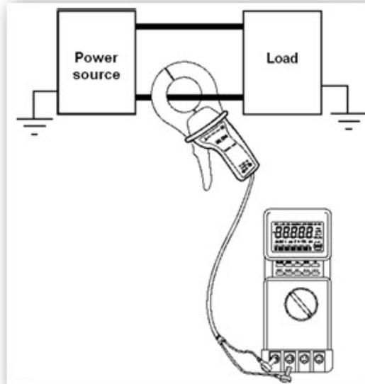
The following AC and DC probes can be used in this setup:
