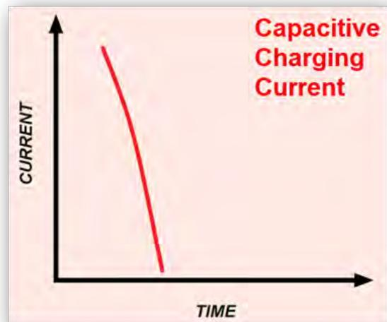
When two conductors are in close proximity separated by an insulator – for example, a length of common two-wire electrical cord -- they can act as a capacitor.
