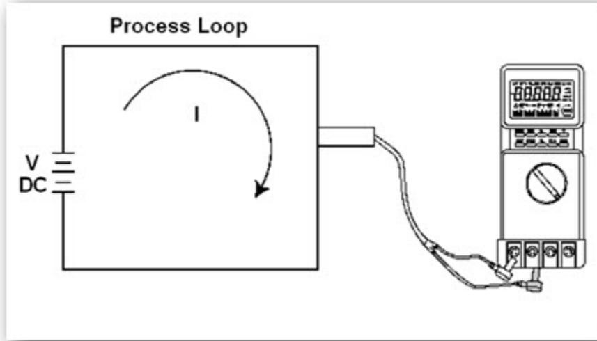
For example, the following probe can be used in process loops:
