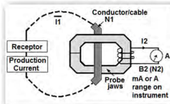
It is often difficult to measure  $I_1$  directly because of currents which are too high to be fed directly into a meter or simply because breaking into the circuit is not possible. To provide a manageable output level, multiple turns are set into the probe coil bobbin.
