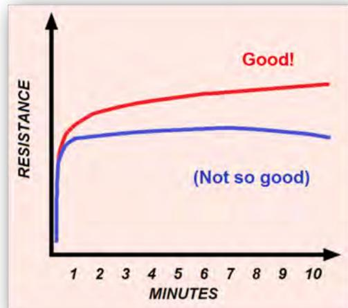
When you plot the results, you should see a curve that rises relatively rapidly at first, and then continues to gradually rise throughout the testing period. If instead the curve is relatively flat or begins to turn down as the test progresses, moisture, dirt, or other factors may be compromising your insulation.
