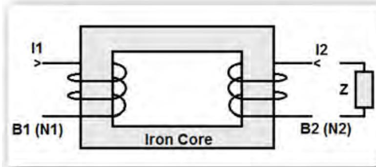
A current  $I_1$  is applied through the coil  $B_1$ , inducing through the common iron core a current  $I_2$  in the coil  $B_2$ .
