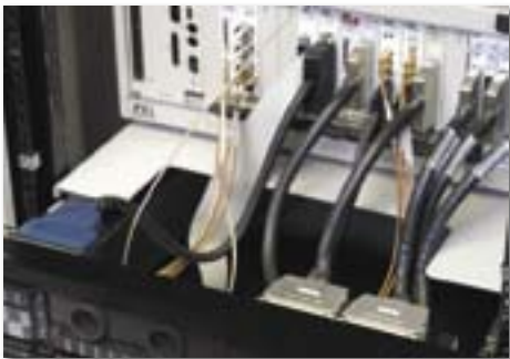
Rapid Integration With PCB Adapters To SCSI, D-SUB, VHDCI, And Other COTS Connectors
