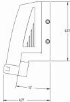
10 Module Interchangeable Test Adapter (ITA) with Sliding, Removable Cover - P/N 410 104 272 10 Module Interchangeable Test Adapter (ITA) with Sliding, Removable Cover and PCB capability - P/N 410 104 270
