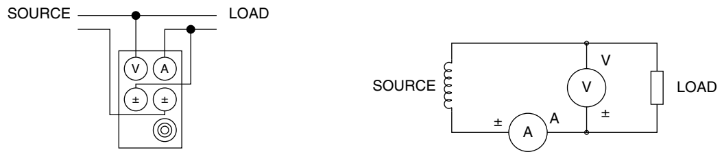
Figure 3-7 Single-Phase, Two-Wire Wiring Schematic
