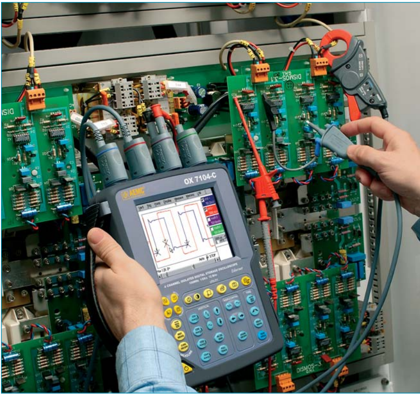
Field testing is quick and easy thanks to the Model OX 7104-CK's hand strap and the use of PROBIX Smart Probes, some that have control buttons, with user definable functions, right on the probes themselves.
